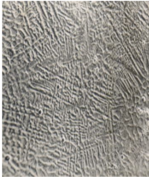
Fig. 3. Microstructure of the weld metal, where they were used as filler electrodes OZCH-2
