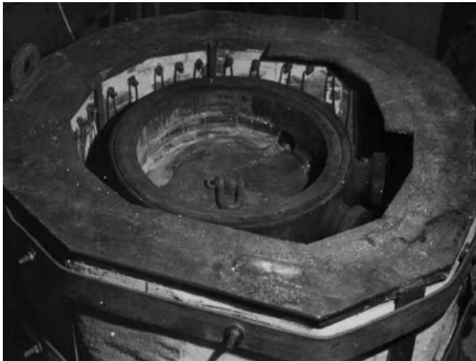
Fig. 7. MAN diesel engine cover placed in an electric heating furnace. Exterior of the repaired cover
