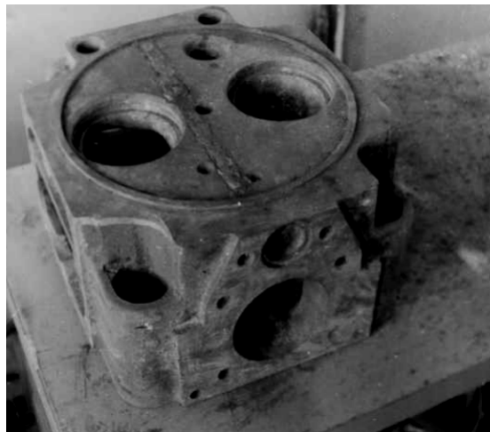
Fig. 5. Cover 6CH25-34 with welded seam
