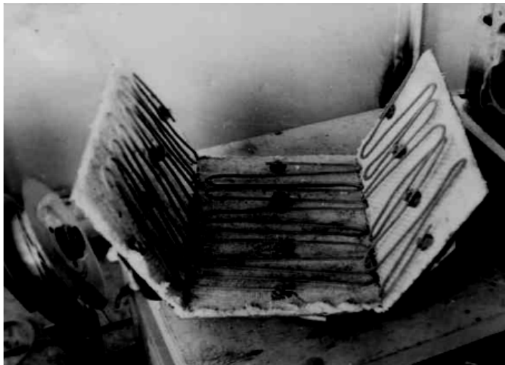
Fig. 9. Electric furnace for heating cast iron piston heads
