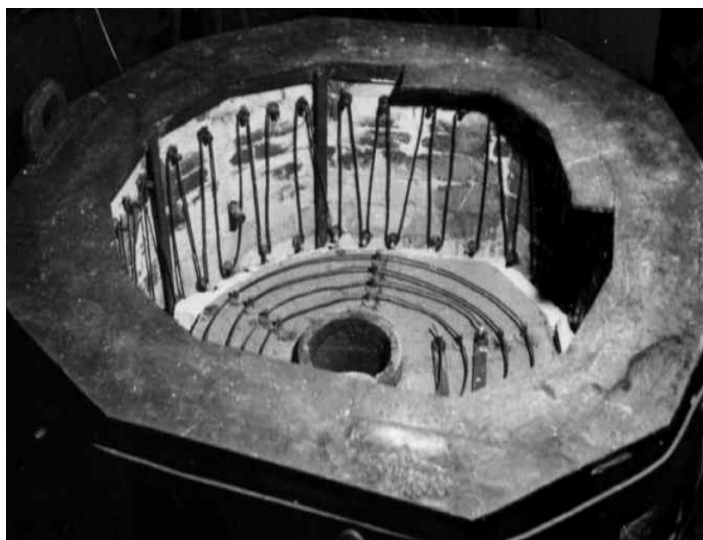
Fig. 1. Electric heating furnace for MAN K6Z57/80F diesel engine covers (cover removed)
